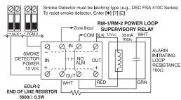
Compatible 4-wire Smoke Detector DSC FSA-410C Series
