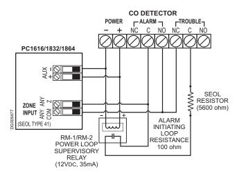
PC1616/1832/1864 v4.5 control panels support operation of 4-wire CO detectors and DSC wireless CO detectors.
